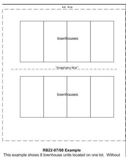
the "imaginary line" between the two rows of townhouses, there is no code provision requiring protection of openings in the walls that face each other
