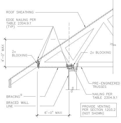
a. Methods of bracing shall be as described in Section 2308.9.3 method 2, 3, 4, 6, 7 or 8
