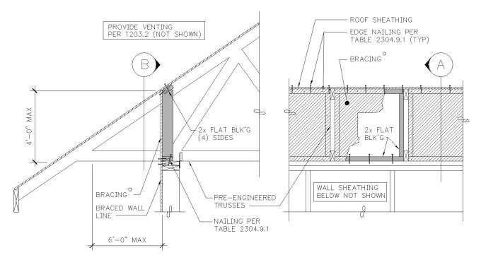
a. Methods of bracing shall be as described in Section 2308.9.3 methods 2, 3, 4, 6, 7 or 8
