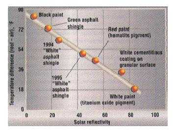
Solar reflectivity is measured according to ASTM E903. Traditional roofing materials have an SRI of between 5% (brown shingles) and 20% (green shingles). White shingles with SRI's around 35% where popular in the 1960's, but they lost favor because they get dirty easily. The trend is to make white shingles more reflective.
