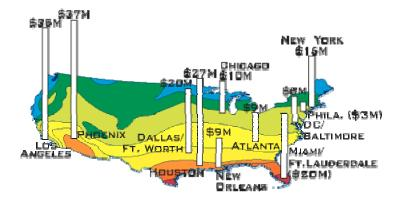
Potential net energy savings from changing roof reflectivity. Savings are measured in dollars. The net savings are the savings of cooling energy use less the penalties of heating energy use.
