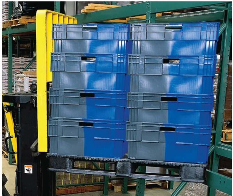
Goods stored on plastic pallets that are listed and labeled as meeting UL 2335 are allowed to be treated as goods stored on wood pallets, for rack storage of commodities. (Photo courtesy of Buckhorn Incorporated.)
