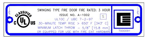
Another issue of concern is a statement in the code that says: "Smoke and draft control doors complying with UL 1784 shall be labeled as such." You will note on the label on the label that the letter "S" appears in a box. This is a shorthand method of indicating compliance to that requirement. This needs to be reflected in the code.
