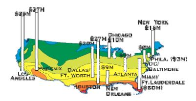
Potential net energy savings from changing roof reflectivity. Savings are measured in dollars. The net savings are the savings of cooling energy use less the penalties of heating energy use.
