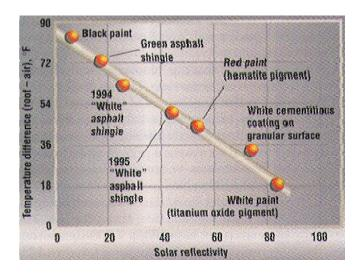
Solar reflectivity is measured according to ASTM E903. Traditional roofing materials have an SRI of between 5% (brown shingles) and 20% (green shingles). White shingles with SRI's around 35% where popular in the 1960's, but they lost favor because they get dirty easily. The trend is to make white shingles more reflective.
