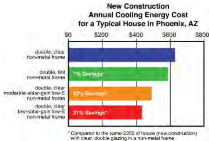
The third graph shows the effects of low solar gain glass (windows with an SHGC at or below 0.25) exclusive of frame (since windows are rated by NFRC with the frame, a 0.27 SHGC glass translates to a whole product SHGC below 0.25). Note that while glass can provide high visible light with low SHGCs, there are also alternatives that provide considerably lower visible light to reduce glare, along with a low SHGC, depending on the occupant's priorities.
