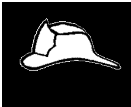
FIGURE 3007.7.5 FIRE SERVICE ACCESS ELEVATOR SYMBOL
