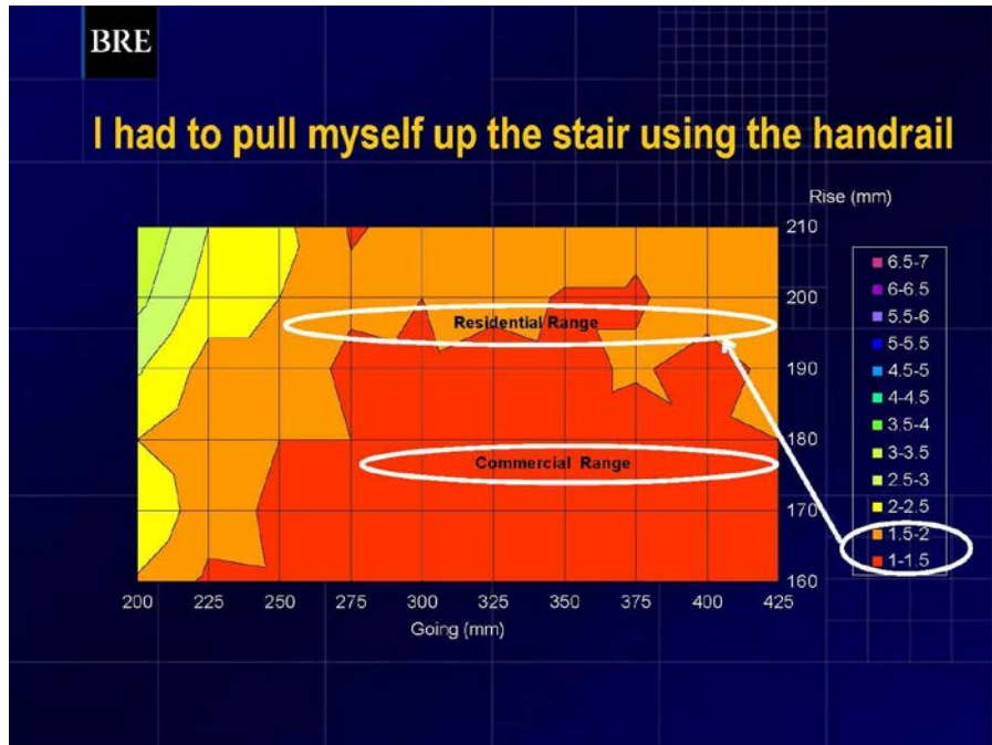
Figure 2 Residential Range = 7.58" (193mm) – 7.74" (197mm), Commercial Range = 6.84" (174mm) – 7" (178mm) see Table 1 Please note that the described circled ranges have been added to figures 1&2 by the proponent for the purpose of explanation.
