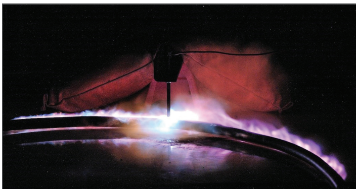
Dissipating Arcing Energy within Arc-Resistant Jacket
