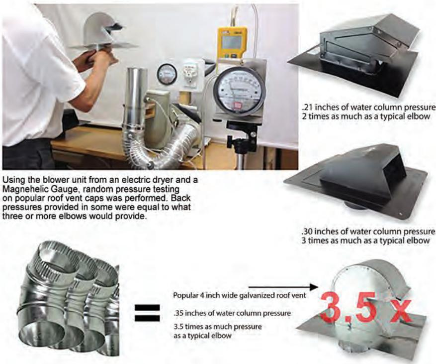
Dryer duct terminals must provide a minimum opening of 12.5 square inches.
