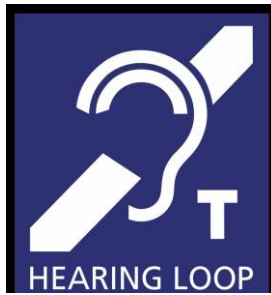
FIGURE 703.6.3.3(A) International Symbol of Access for Hearing Loss with a “T” to indicate a hearing loop
