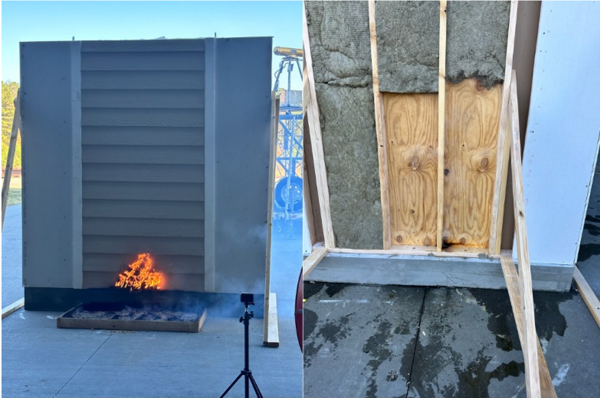
Figure 3. a. 1-hr FRR assembly with unprotected OSB Sheathing material at the bas3. Photo curtesy by Milad Shabanian, IBHS.
