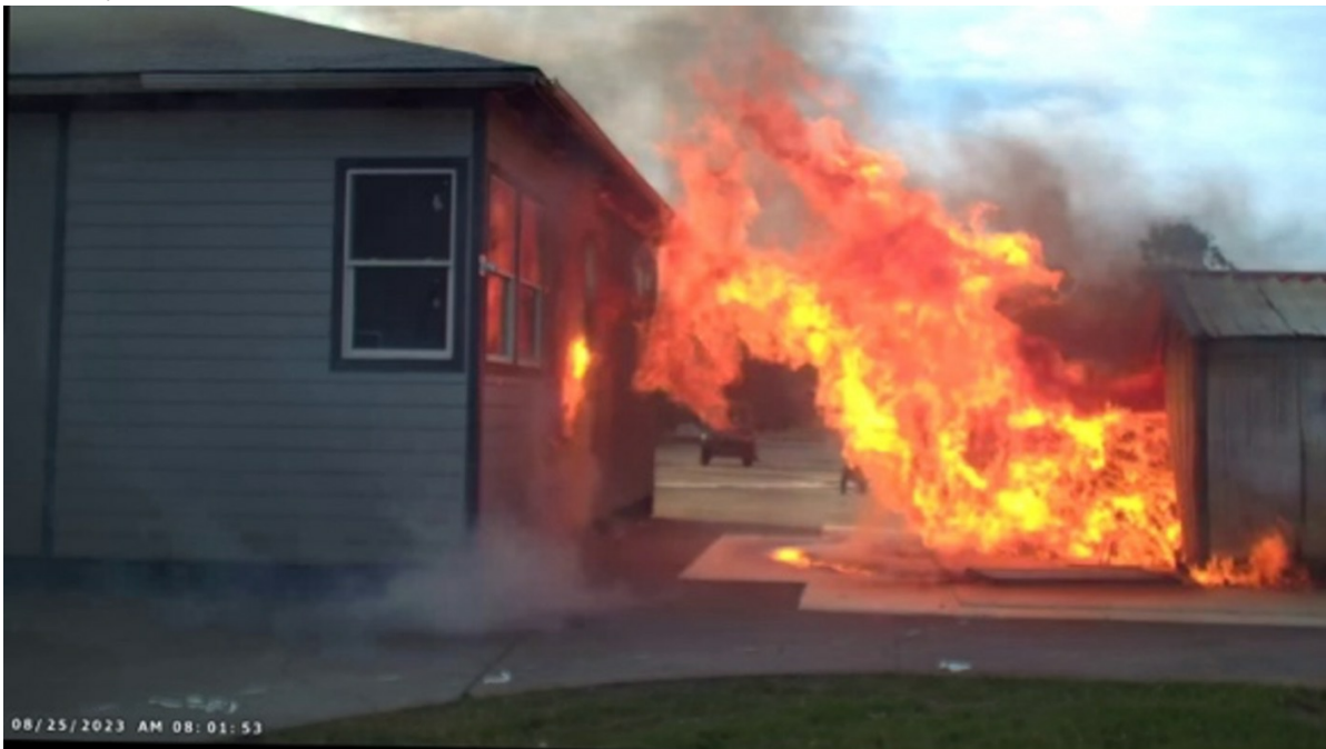
Figure 1. b. ignition of the combustible siding.
