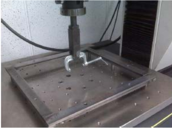
Test machine fixtures for the pull-through test.
