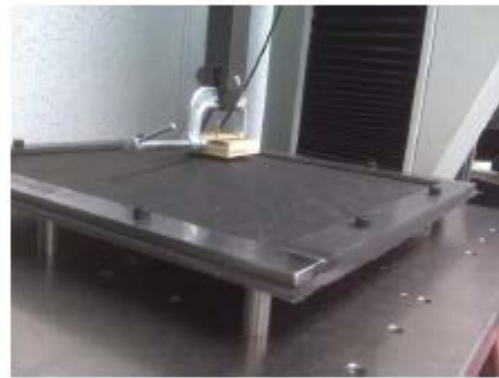
Pull-through test in progress; (left) early in test; (right) nearing failure.
