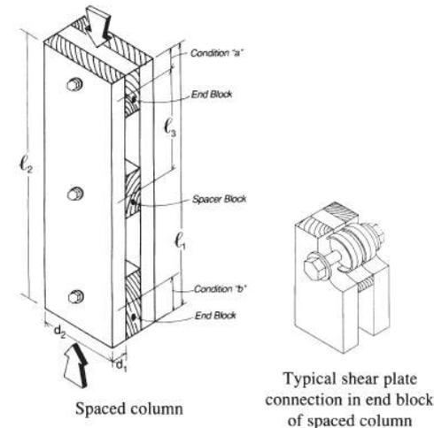
**Figure 15B Mechanically Laminated Built-Up Columns**
