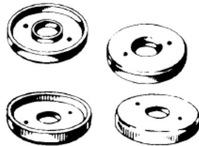
**Figure 13C Malleable Iron Shear Plate Connector**
