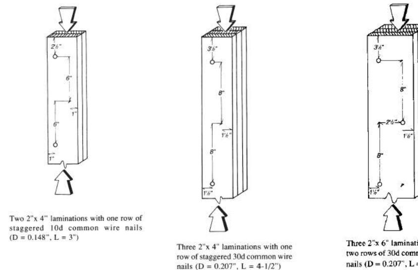
**Figure 15E Eccentrically Loaded Column**
