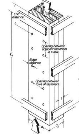
**Figure 15D Typical Bolting Schedules for Built-Up Columns**
