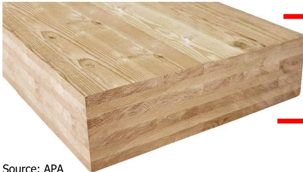
→  $EI_{eff}$  = Effective bending stiffness of the CLT section, lbs-in.<sup>2</sup>/ft of panel width
