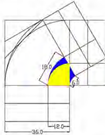
Figure 3: The 60 and 90 degree landings are shown superimposed. The total area inside of the walk line of the 60 degree winder is clearly comparable to that of conventional landings when the suggested minimum dimensions are applied.
