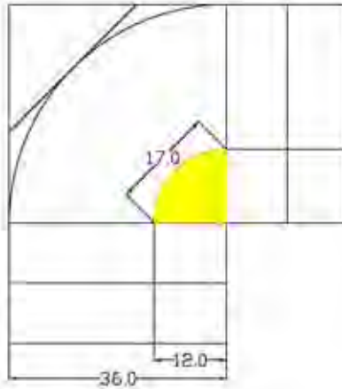
Figure 2: Conventional 90 degree Landing. The total area inside of the walk line is shaded.
