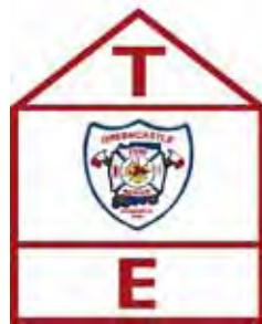
FIGURE 316.6.2 EXAMPLE STRUCTURAL IDENTIFICATION LABEL
