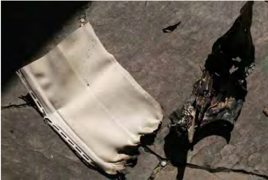
Figure 2 Polypropylene siding melting and flaming on the floor. (No figure 2 attached)
