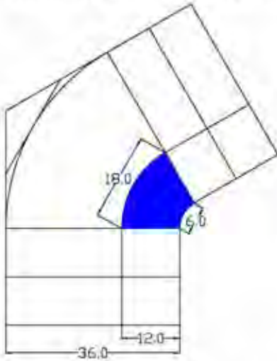
Figure 1: Proposed 60 degree minimum Landing. The critical area inside of the walk line is shaded.
