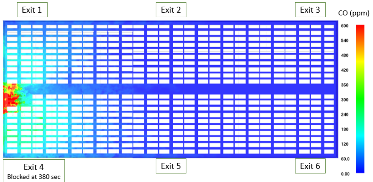
Figure 5-13. CO concentrations 6 ft above the floor at RSET (904 sec (15.07 min)) for west wall fire location
