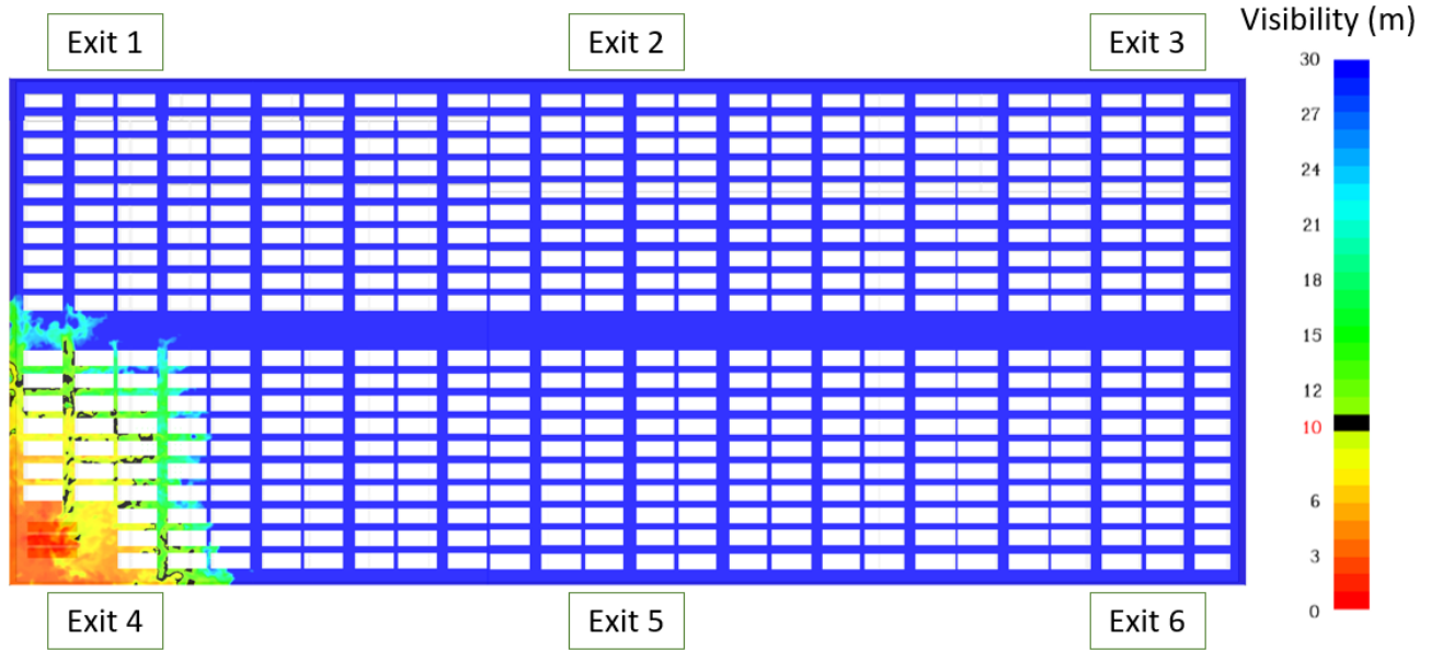
Figure D-9. Visibility conditions 6 ft above the floor at 180 sec (3 min) for southwest corner fire location
