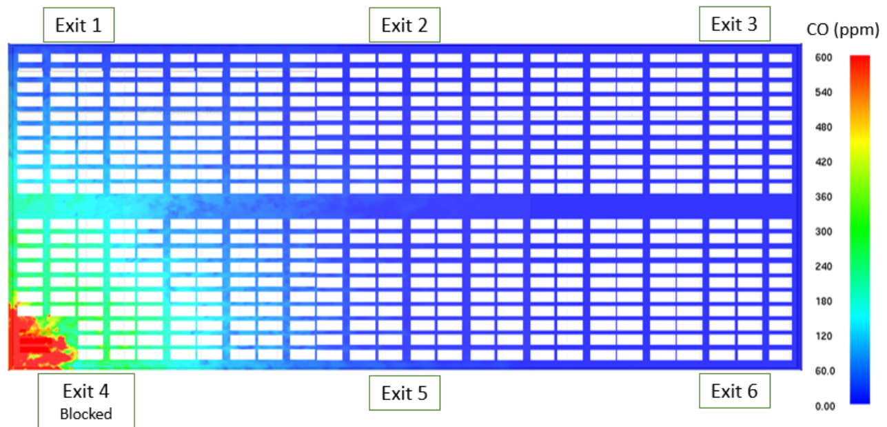
Figure 5-9. CO concentration 6 ft above the floor at RSET (847 sec (14.1 min)) for southwest corner fire location
