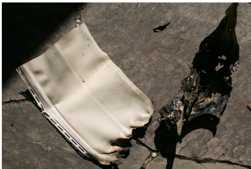
Figure 1 – Remains of vinyl siding fire
