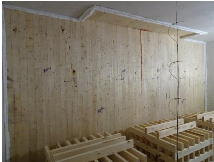
Figure 24. CLT room with Wall A and 10% ceiling exposed for Test 2.
