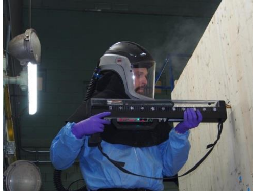
Figure 31. A Resistograph drill used to determine CLT char depth after Test 2.
