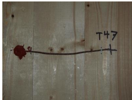
(b) 150 mm wire run along CLT interior surface
