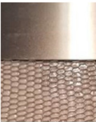
Figure 1. Metal honeycomb core (facing removed on lower half) – Combustible adhesives used to attach both top and bottom facings.
