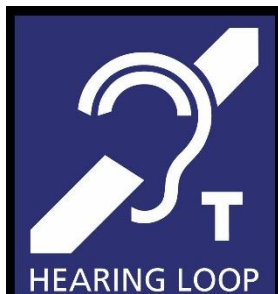
FIGURE 703.6.3.3(A) International Symbol of Access for Hearing Loss with a “T” to indicate a hearing loop
