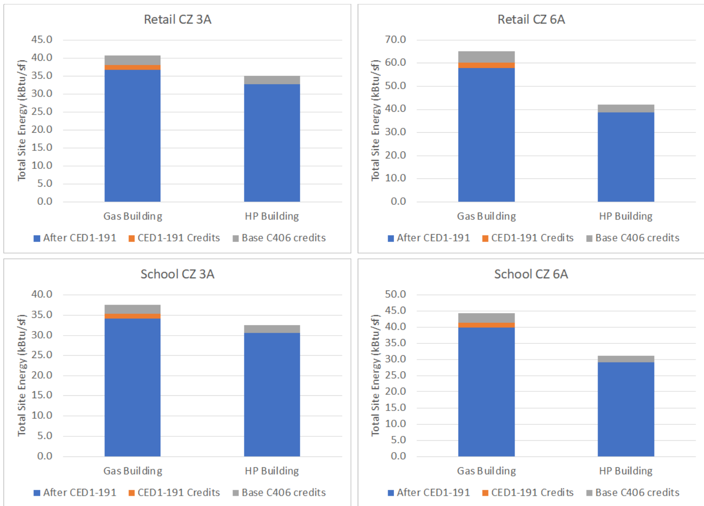
Fig. 1: Comparing site EUI of fossil fuel and electric heat pump buildings using DOE prototype models
