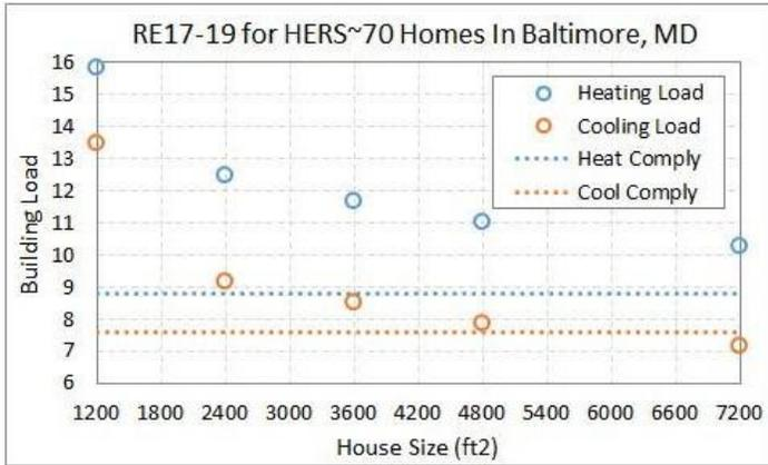
Notes: Insulation values approximately equal to 2012 IECC. HERS Index score of 70 based on RESNET/ICC 301. None of these homes fully comply with RE17-19, but it's clear that larger homes will have an easier time complying than smaller homes.
