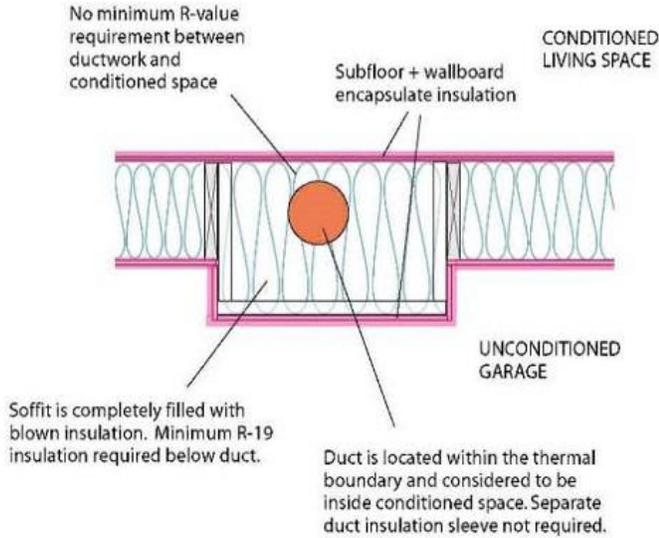
NOTE: This approach is only approved if BLOWN insulation is used to completely fill the soffit.
