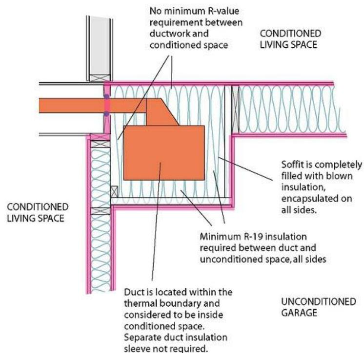
NOTE: This approach is only approved if BLOWN insulation is used to completely fill the soffit.
