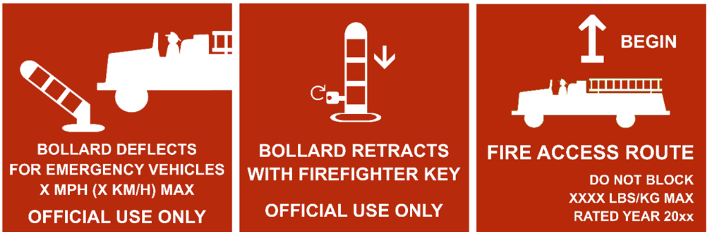
FIGURE D105.2.2.6 EXAMPLES OF SIGNS AND GROUND TILES FOR MARKING WORKING AREAS
