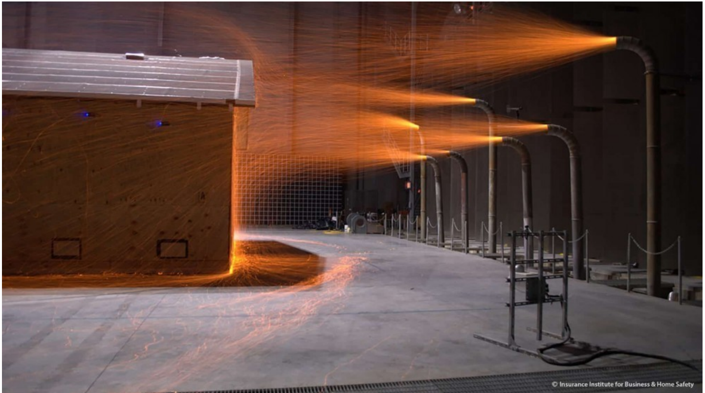
Photo shows IBHS research on vent intrusion from embers.
