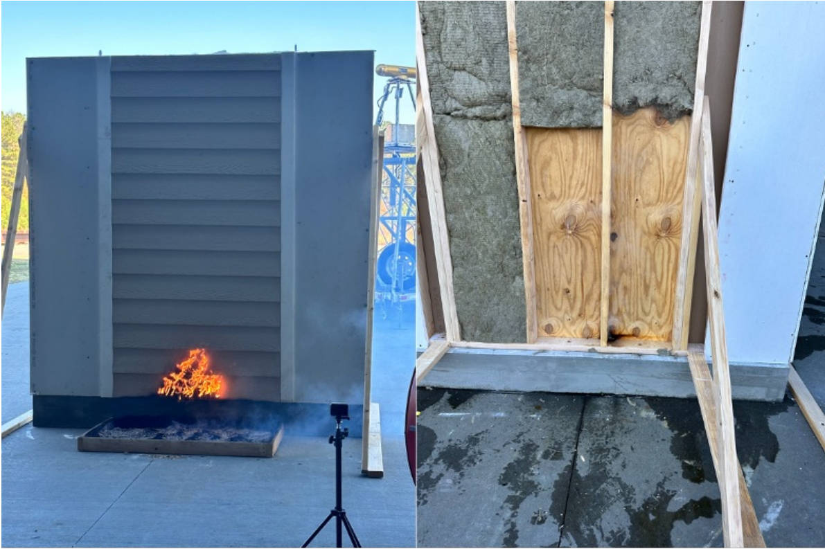
Figure 3. a. 1-hr FRR assembly with unprotected OSB Sheathing material at the bas3. Photo curtesy by Milad Shabani, IBHS.
