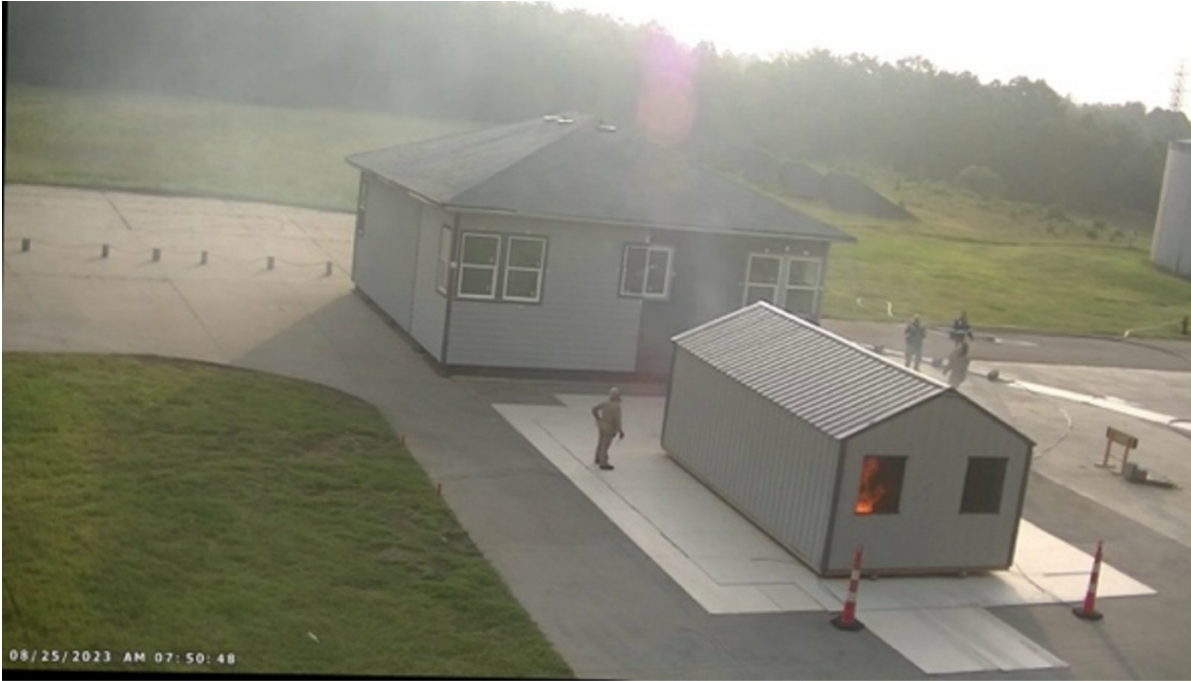
Figure 1. a. The test setup for wind driven building to building fire spread tests. The target building has an hour fire resistant rated wall assembly.
