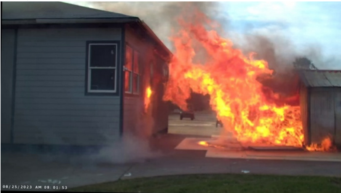
Figure 1. b. ignition of the combustible siding.
