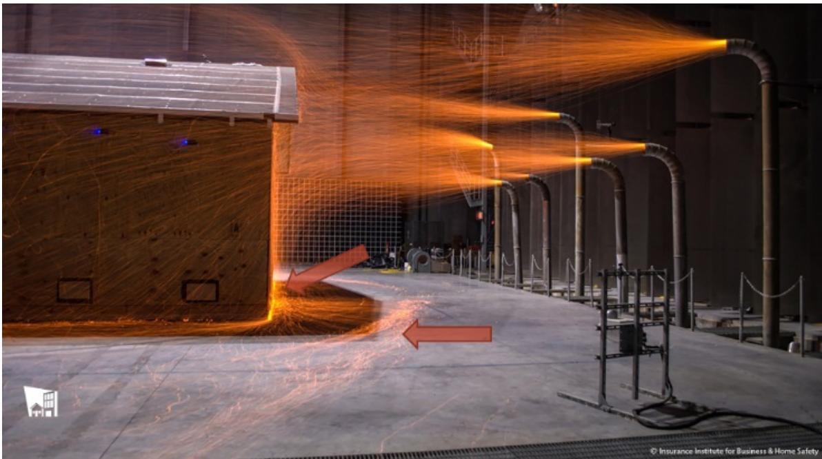
Figure 4. Ember accumulation around a building, IBHS Research Center.
