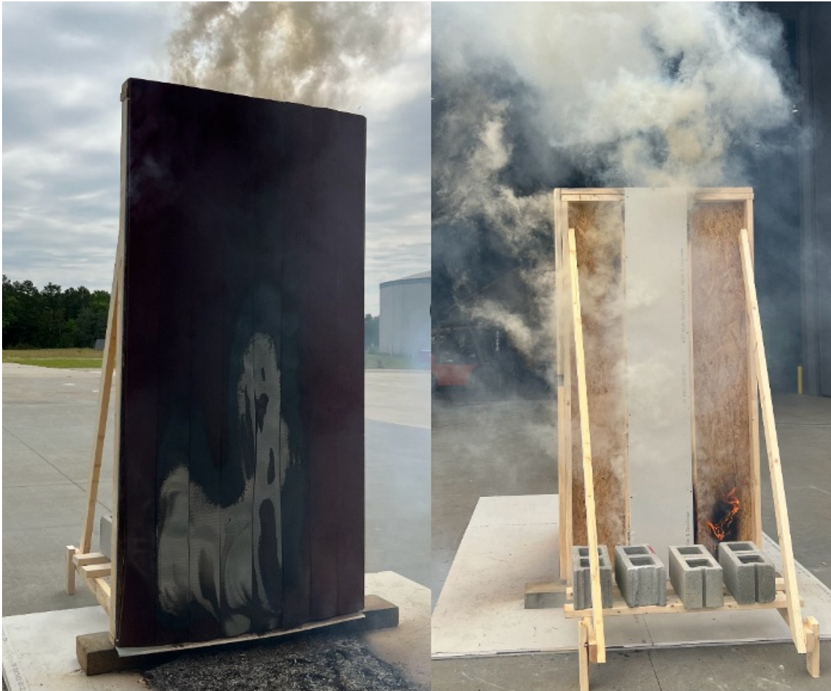
Figure 4. a. Typical exterior wall assemblies constructed on the exterior with noncombustible metal siding. Photo courtesy by Milad
