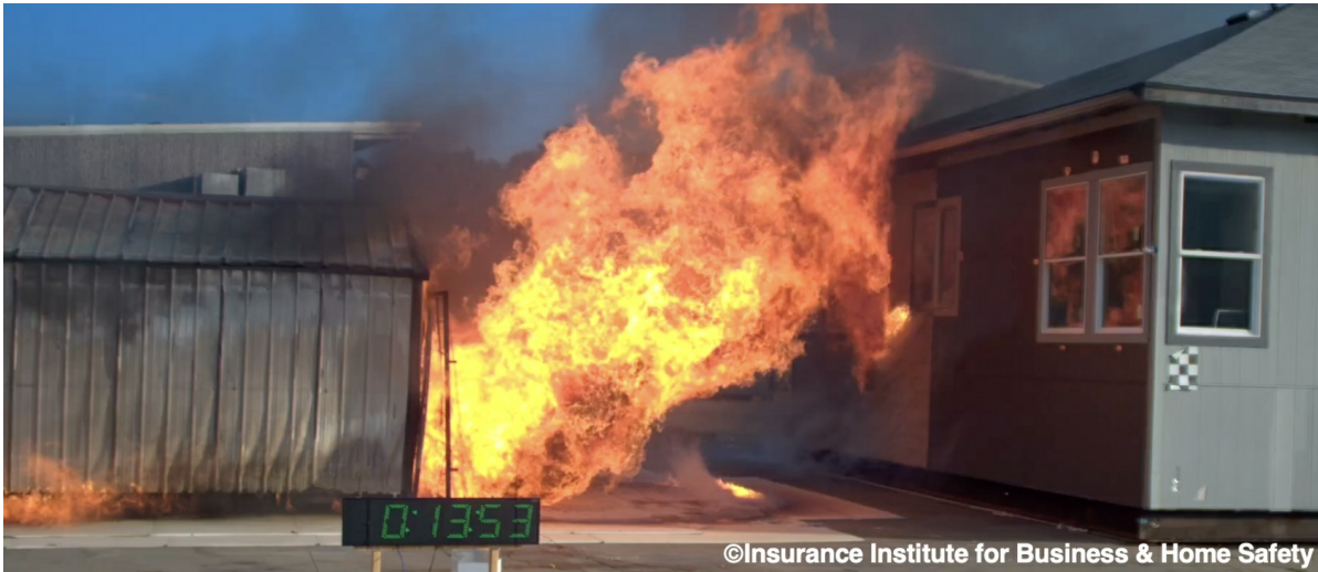
Figure 1. Possible fire exposure to target structure caused by noncombustible detached accessory structures 20 ft away from target structure.
