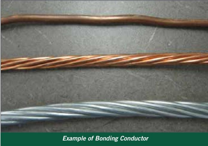
Example of Bonding Conductor
