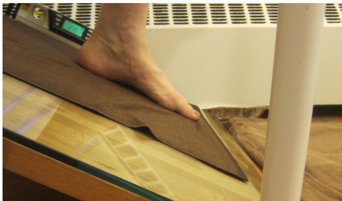
Fig. 5. 27.5-degree ( \tan 0.52 ) slope glass ramp surface with damp terry cloth towel showing slow creep just beginning.
