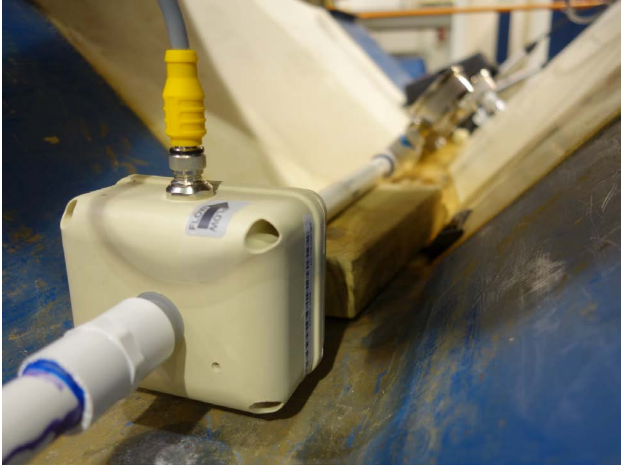
Figure 2. Test apparatus showing flowmeter (credit Michael Gutierrez UF/IFAS)
