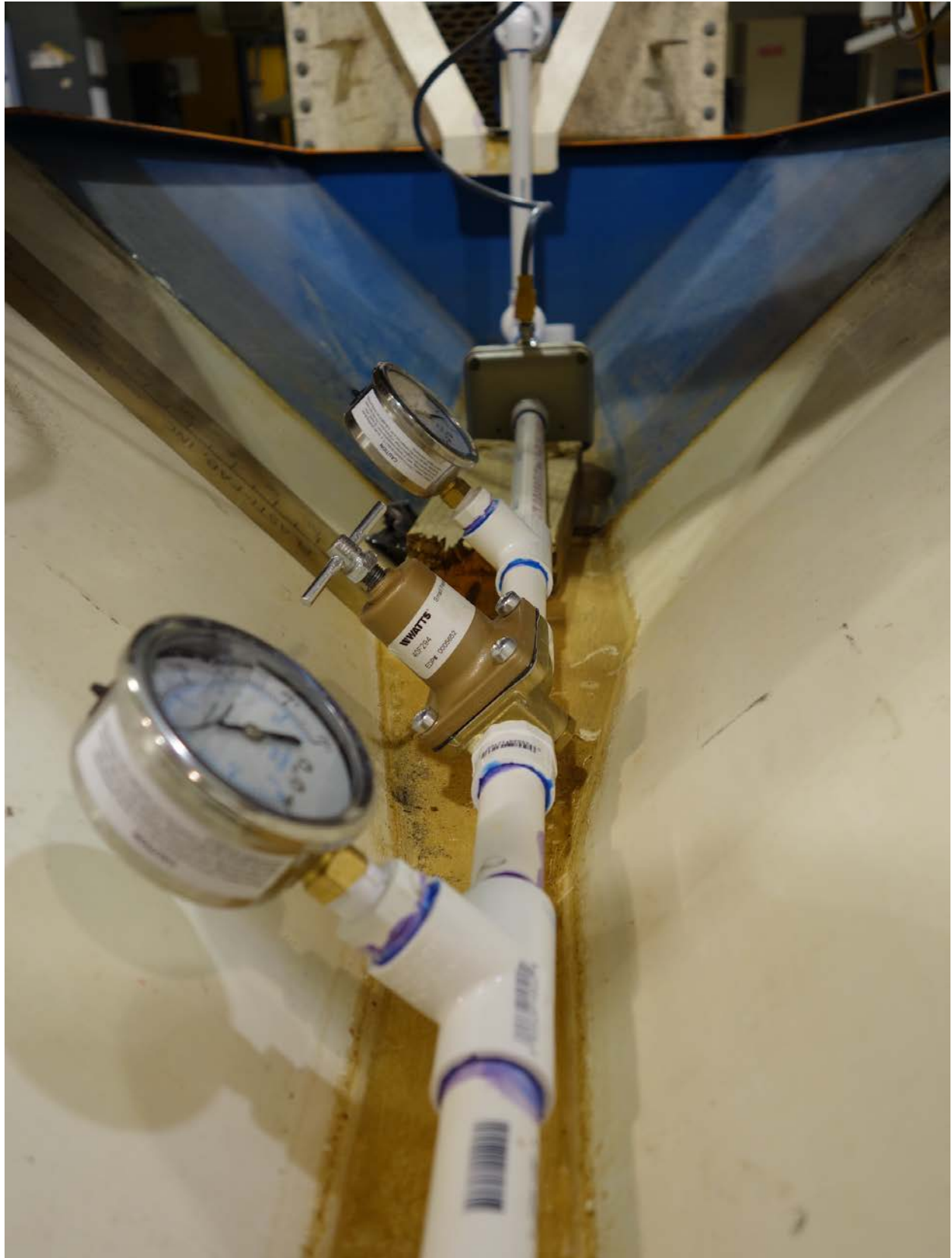
Figure 4. Adjustable pressure regulator and pressure gauges (credit Michael Gutierrez UF/IFAS)
