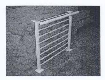
Test Barrier No.2b – Same as barrier 2a (1.0 metre height) with horizontal rails spaced with no opening exceeding 100mm. Top of barrier with an inward return of 200mm (with no opening exceeding 100mm).
