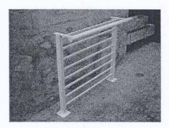
Test Barrier No.3a – Barrier at 1.0 metre height with no toeholds between ground and 610mm (with no opening exceeding 100mm), and horizontal rails above 610mm.
