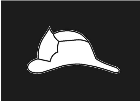
FIGURE 3007.7.5 FIRE SERVICE ACCESS ELEVATOR SYMBOL
