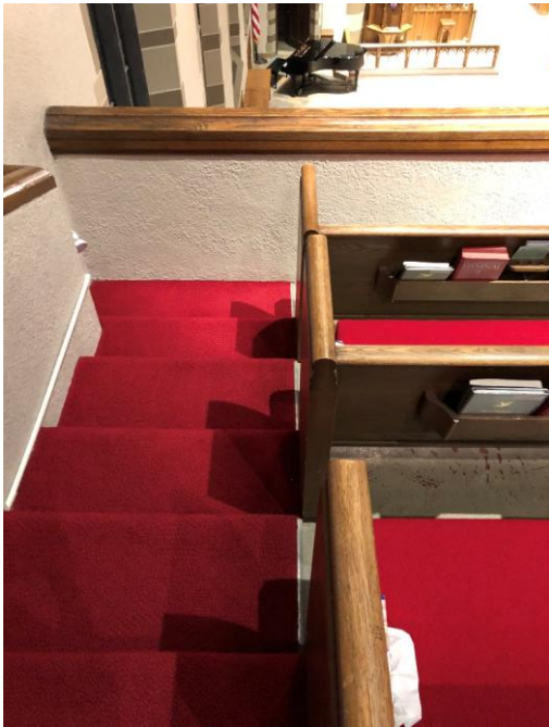
Figure 6 First United Methodist Church in Kalamazoo, MI Handrail built into end of pew. Stepped aisle with seating on one side. The knob dimensions sited are common for door knobs.
